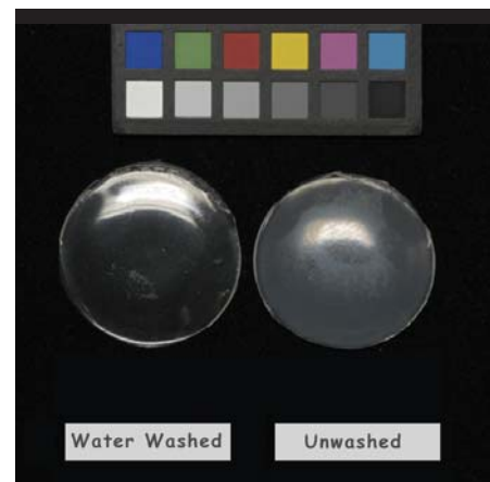
Figure 2: Surfactant Exudates - pours of acrylic dispersion polymer. Right: untreated pour; Left: pour washed/soaked with water. After 2 weeks of drying, this pour was soaked in water for 10 minutes, then dried.
