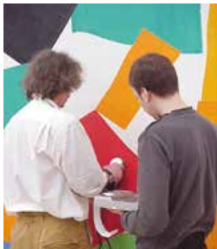
Tate's expert conservators used a spectrophotometer to monitor the colour density of each layer of the work.
