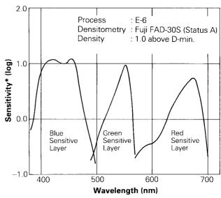
Sensitivity equals the reciprocal of the exposure (erg/cm²) required to produce a specified density.
