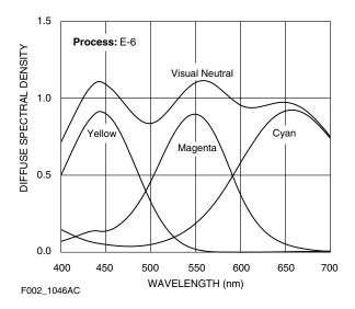
These curves depict the spectral absorptions of the dyes formed when the film is processed. They are useful for adjusting or optimizing any device that scans or prints the film.
