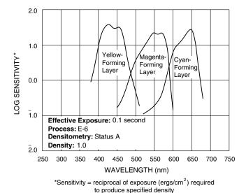
These curves depict the sensitivity of this film to the spectrum of light. They are useful for determining, modifying, and optimizing exposure for blue- and green-screen special-effects work.
