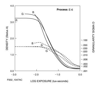
To find the rms Granularity value for a given density, find the density on the left vertical scale and follow horizontally to the characteristic curve and then go vertically (up or down) to the granularity curve. At that point, follow horizontally to the Granularity Sigma D scale on the right. Read the number and multiply by 1000 for the rms value. Note: This curve represents granularity based on modified measuring techniques. A slight variation from sensitometric curve may be noticed.
