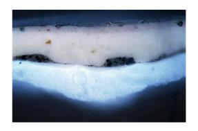
Figs.3a and 3b Cross-section showing single ground (lower semi-transparent layer with thin 'flatting' coat on top) plus grey and off white paint layers. Incident light (left) and ultraviolet light (right). Photographed at 250x.
