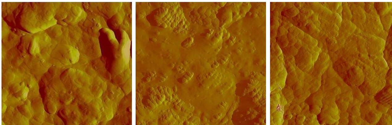
*AFM image (10 x 10µm) of Talens titanium white test film (high levels of surface surfactant).
