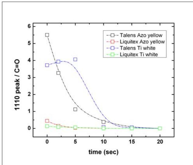
*Monitoring the aqueous removal of PEO-based surfactants from the surface of four test acrylic emulsion films on canvas with FTIR-ATR spectroscopic analysis. Liquitex and Talens titanium white (PW6) and azo yellow (PY3) test films. © Tate 2009.*
