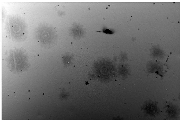
*A back-scattered electron scanning electron microscopy (BSE-SEM) image (100x) of the surface of a Winsor and Newton titanium white test paint film.*
